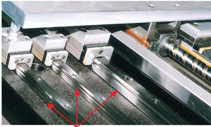
NSK K1™ installed linear guide
