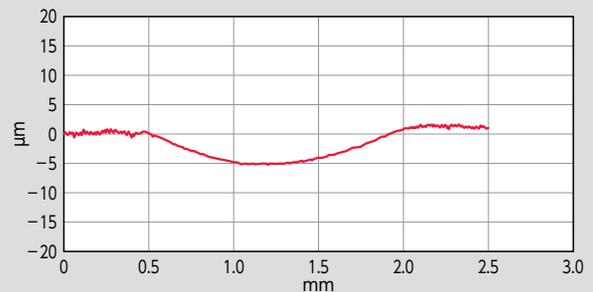
Abrasion around 5 to 6 µm
