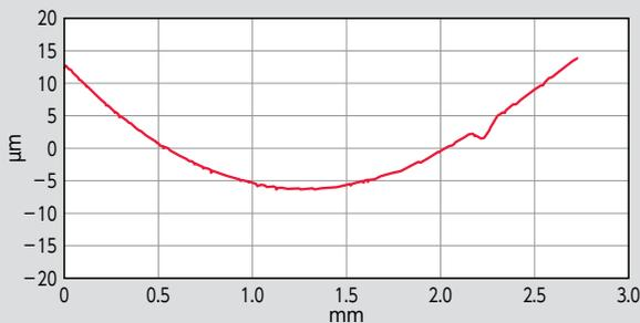
Abrasion higher than 20 µm
